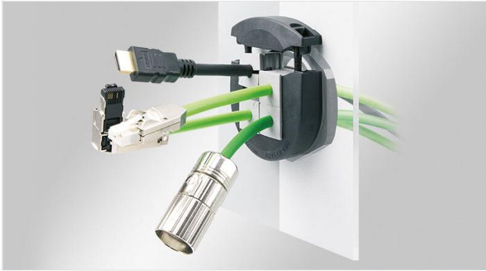
KVT-ER are split cable glands for routing and sealing cables with connectors, with diameters from 1 to 16 mm (KT 1 - 15) and 16 to 35 mm (KT 16 - 34). But also electric, pneumatic or hydraulic lines without terminals or connectors as well as corrugated conduits can be easily routed (e.g. into control panels, enclosures or machinery), sealed and strain relieved acc. to EN 62444.
