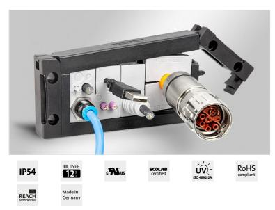
The KEL-FA range is a compact system to route and seal pre-terminated cables as well as conduits or pneumatic hoses utilising KT series <u>grommets</u>. After populating the entry frame with grommets and cables, the cover is put on and the two clamping levers are locked with the lower part by pressing them down. The twist-proof construction of the KEL-FA enables intuitive assembly. Routing and sealing with IP54 / UL Type 12 for cable diameters from 1 to 35 mm.
