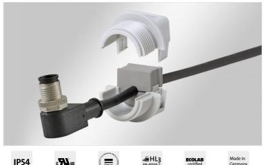
QVT is a circular split frame for quick and easy installation of pre-terminated cables or complete cable harnesses. But also electric, pneumatic or hydraulic lines without terminals or connectors as well as corrugated conduits can be easily routed and sealed with IP54. Because of its extremely compact design, the QVT range is especially suitable for small machines, devices and instruments.
