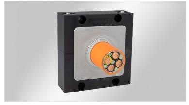
The KEL-JUMBO cable entry system for installation of cables and conduits with a diameter of up to 65 mm, especially suited for supply cables. The innovative grommet design with the flex-membrane provides flexing and adjustment of the position for larger and more rigid cables.
