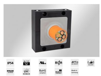
The KEL-JUMBO cable entry system for installation of cables and conduits with a diameter of up to 65 mm, especially suited for supply cables. The innovative grommet design with the flex-membrane provides flexing and adjustment of the position for larger and more rigid cables.
