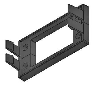
42061 Part No. Cut-out size 86 × 36 mm EAN **4251269323** No. of screw 737 holes Package 10 Diam. of screw **5,5 mm** quantity holes Length 128 mm Suitable for KEL 16, KEL-Width 64 mm cable entry U 16, KEL-FA 16, KEL-Height 38 mm systems: 38 mm **QUICK 16** Mounting
