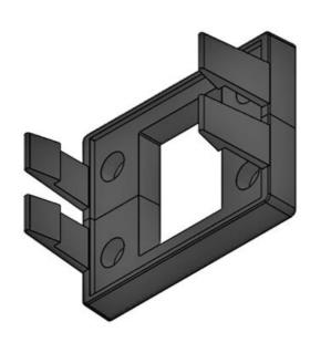
Part No. 42063 Cut-out size 46 × 46 mm EAN 4251269323 No. of screw 751 holes Package 10 Diam. of screw 5,5 mm quantity holes Suitable for 81 mm KEL-B, KEL-Length Width 64 mm U-B, KELcable entry Height 38 mm QUICK-B systems: Mounting 38 mm Split Yes
