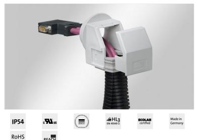
The split KVT-W90 cable glands are used to insert and seal pre-terminated cables at a 90° angle. But also electric, pneumatic or hydraulic lines without terminals or connectors as well as corrugated conduits can be easily routed (e.g. into control panels, enclosures or machinery) and sealed with IP54.
