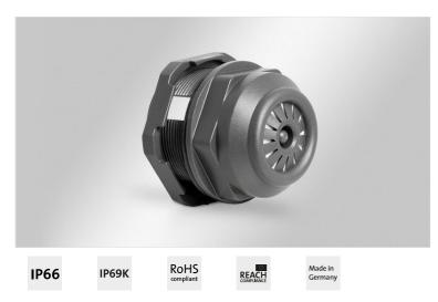
In enclosures and housings with a high degree of protection, temperature differences result in condensation. By using a drainage device, it is possible to safely drain off the condensate without losing a maximum enclosure protection of IP66. A water-permeable membrane ensures the drainage of the enclosure due to its capillary effect. The design prevents splash water from entering the interior of the enclosure.
