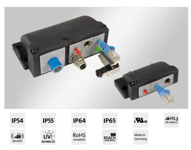
The cable entry frames KEL-FG-ER are suited for installation of cables with connectors and conduits at an angle of 90° to the cabinet, enclosure or machine wall, providing an IP65 rating and strain relief for cable diameters from 1 to 16 mm (single-hole grommets KT 1 - 15) and 13 to 35 mm (single-hole grommets KTG 13 - KT 34).
